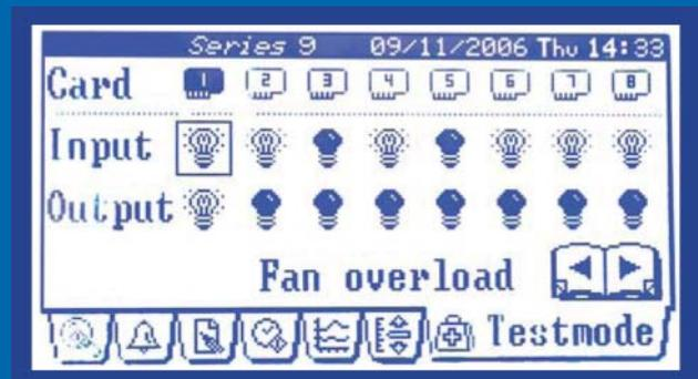
**I/O BOARD DIAGNOSTIC FOR UNIT IN CO-WORK™ NETWORK - SCREEN 2**
